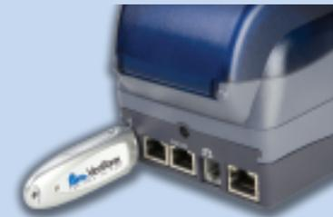
*USB port allows for easy, secure application downloads from a Flash memory drive.*
